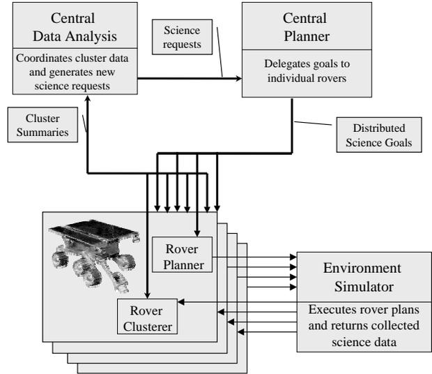
Figure 1: MISUS Architecture Diagram
